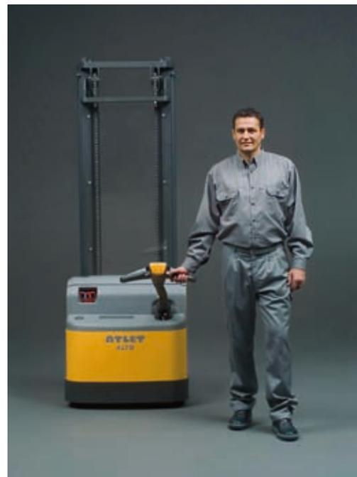
The position of the tiller arm makes it easy to operate the truck while walking beside it.
