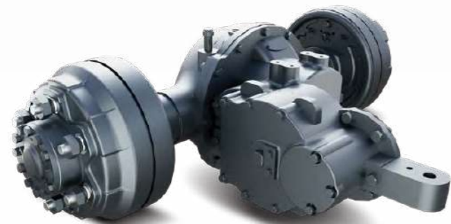
Drive axle: integral brake drum, integral cast axle housing, half shaft oil seal design, high-precision gear with large coincidence
