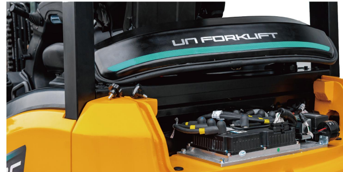
Fully opening engine cover for easy maintenance of the battery and hydraulic pump motor.
