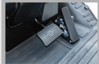
Hanging foot brake achieve smooth braking and reduce vibrations.
