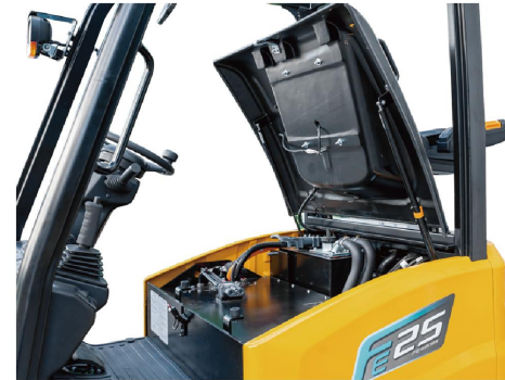
Fully opening engine cover for easy maintenance of the battery and hydraulic pump motor.
