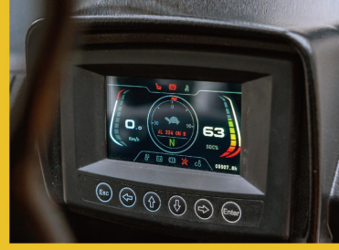
Multi-function color screen instrument provides key information of forklift.
