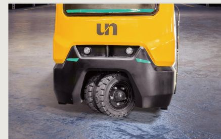
The standard turning speed deceleration function reduces the risk of tipping over in corners.
