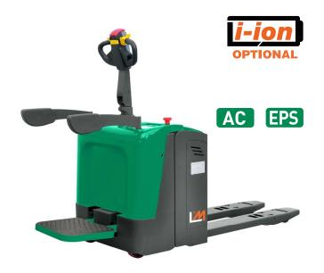
Fast, simple and powerful, but safe and easy-to-use for all your horizontal pallet transport needs in a wide range of light and medium duty applications. The standard Creep speed button ensures high maneuverability in confined areas when operating at low speeds with the tiller in the upright position.
